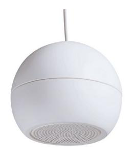
The 16 W powered speaker is equipped with a 130 mm full-range loudspeaker chassis and a 100 V transformer with 3 power adjustments. The sturdy, UV-resistant ABS-housing (UL 94 HB) in RAL 9010 guarantees long-term stability. For additional reliability, a ceramic block, a thermal fuse is provided and the speaker chassis is impregnated against wetness.
