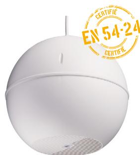
The 20 W powered speaker is equipped with a 165 mm fullrange loudspeaker chassis and a 100 V transformer with four power adjustments. Power adjustments can easily be done by turning a knob at the top of speaker. The operation in low impedance mode is also possible. The sturdy, UVresistant ABS-housing (UL 94 V0) in RAL 9016 guarantees long-term stability. For additional reliability, a 2 pin-ceramic block, a thermal fuse is provided and the speaker chassis is impregnated against wetness.
