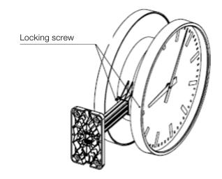
Connect the cables in consol to the clockwork. Mount the clock to the consol by turning in clockwise direction.
